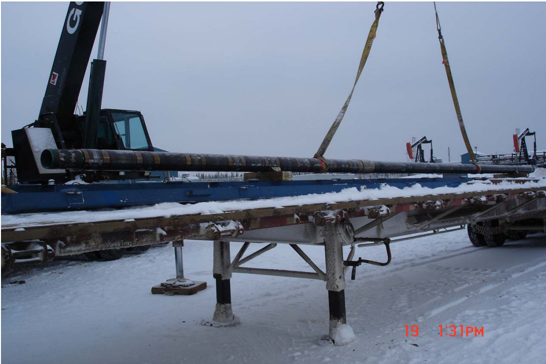
CAN-K PUMP BEING LIFTED TO RIG FLOOR
